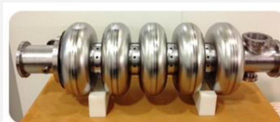
Figure 1: High beta 704.42 MHz undressed cavity.
